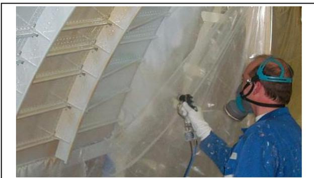
**Using Aerosol Sprays:** ARDROX AV CICs are available in aerosol spray cans, these are very effective for treating small areas, for touchup and for small scale maintenance and repair.
